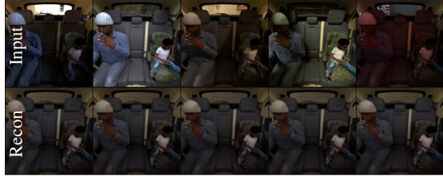
Figure 5: The encoder-decoder model transforms the input images of a same scenery (first row) into a cleaned version (second row) by removing all illumination and environment information (see the background through the window)
